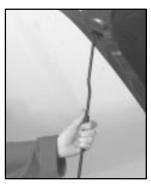
Lift the hood, release the hood prop from its retainer and put the hood prop into the slot in the hood marked "prop rod."
